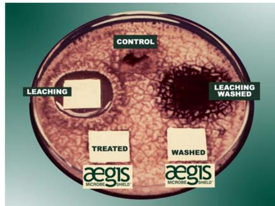
**FIGURE 1 Results: AATCC Method 30; AEM 5700 treatment, conventional antimicrobial treatment, and untreated control. Washed<sup>1</sup> and unwashed.**
